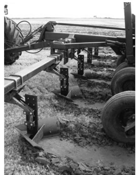
**Figure 8.** The agricultural coulters bar, and five mounted mini-scalping units. The breakout assembly and mounts for each mini-scalp were developed by Danny ten Seldam.
